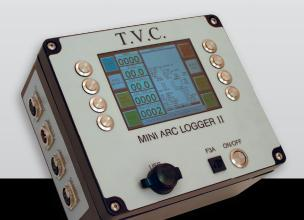
Its 5.7-inch TFT screen provides a clear view of all monitored welding parameters and the sealed battery allows up to eight hours of monitoring time between charge cycles.
